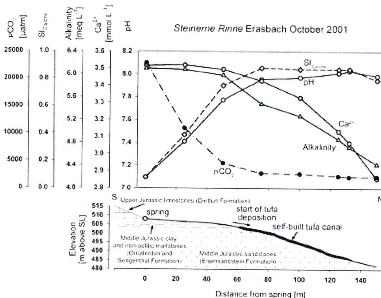
Figure 4. An example of the downstream changes in: CO<sub>2</sub> pressure (pCO<sub>2</sub>), calcite saturation (Si<sub>Ca</sub>), alkalinity, calcium concentration and pH along a travertine deposition stream. The outgassing of CO<sub>2</sub> results in an increase of the pH from about 7 up to 8–8.5. As the outgassing takes some time the precipitation of tufa usually starts somewhat downstream of the spring (after Arp *et al.* 2010).
